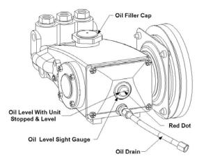
2. After **50 hours** operation, change the crankcase oil with CAT Pump Crankcase Oil, (Part # 13-000). Change the crankcase oil every **500 hours** thereafter.
